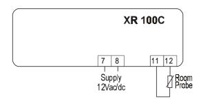
**24Vac/dc:** supply the instrument to the terminals 7 -8. **120Vac:** supply the instrument to the terminals 7 -8. **230Vac:** supply the instrument to the terminals 7 -8.
